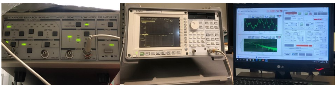
Figure 4. 5 Acquisition signals system components: Voltage preamplifier; Digital Signal Analyser; Computer using application for signal analysis
