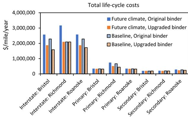
**FIGURE 6** Net present value of the total life-cycle costs of the original binder and upgraded binder under baseline and future climate conditions. Underlying data used to create this figure can be found in the Supporting Information S1
