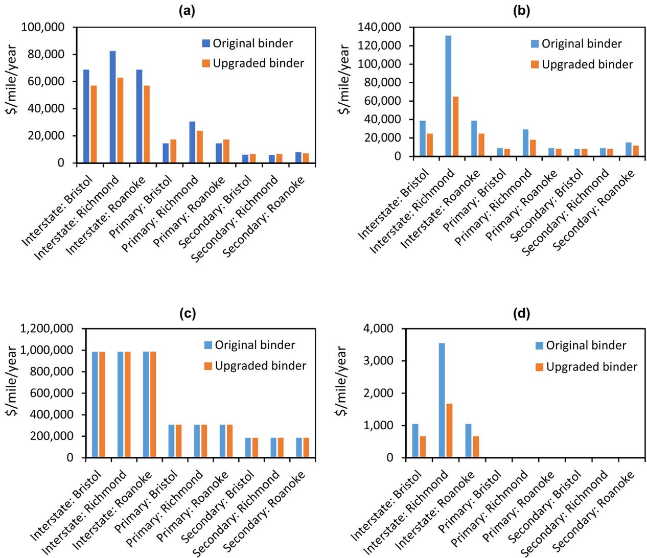
**FIGURE 5** Life-cycle costs incurred during the different phases of the pavement life cycle under future climate: (a) material production phase; (b) maintenance phase; (c) use phase; and (d) work zone phase. Underlying data used to create this figure can be found in the Supporting Information S1
