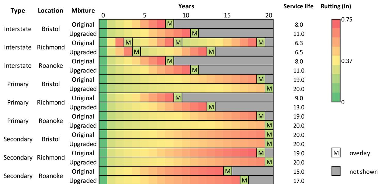
**FIGURE 4** Maintenance interventions and rut depth under future climate conditions. Underlying data used to create this figure can be found in the Supporting Information S1
