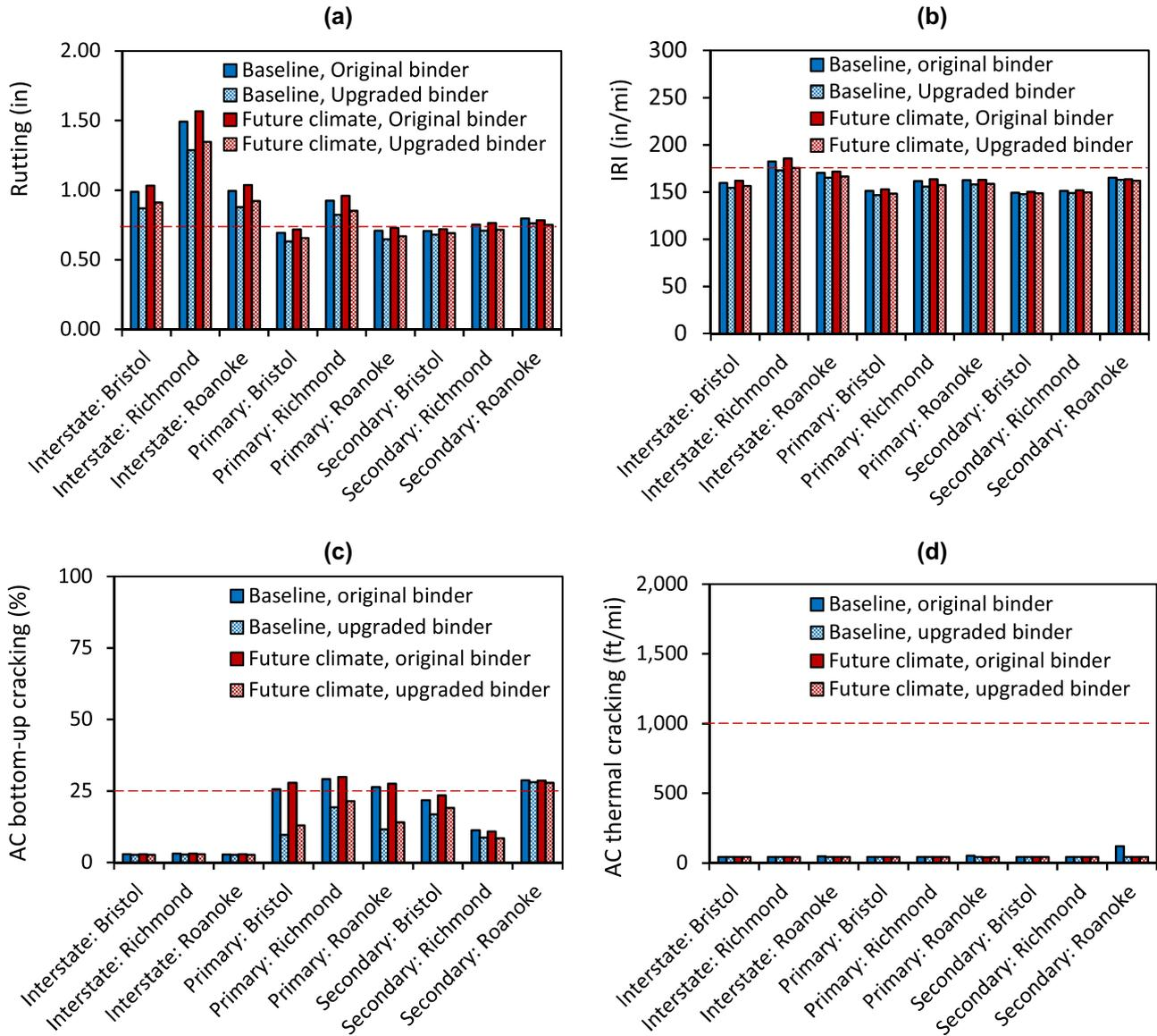
**FIGURE 3** Terminal values of the pavement performance indicators predicted by Pavement ME for the year 20 (the dash lines represent maintenance triggers): (a) terminal rutting; (b) terminal roughness in IRI; (c) terminal asphalt concrete bottom-up cracking; and (d) terminal asphalt concrete thermal cracking. Underlying data used to create this figure can be found in the Supporting information S1
